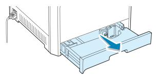
**2** Push down on the metal plate until it locks into position.
